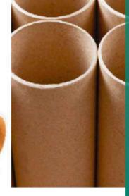
Paper tubes are produced by winding layers of paper using a guide shaft of required diameter.
